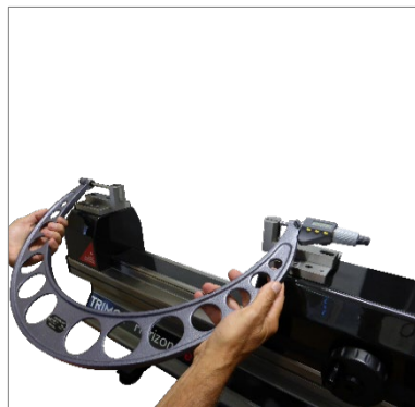
Manually checking of external micrometer (TEL5, TEL 11)
