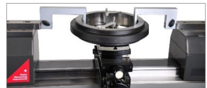
Checking of ring gauges from 12mm
