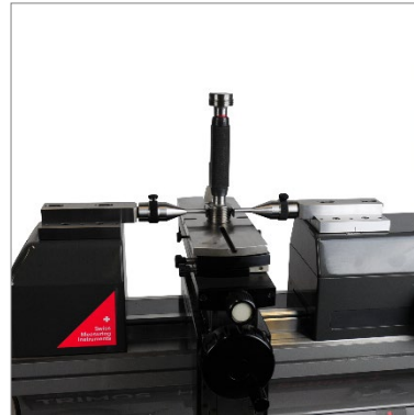
Checking of thread plug gauges (from m100 upwards) (TA-SU-313, TEL6, 3P/0.17-3.2/S6.5)
