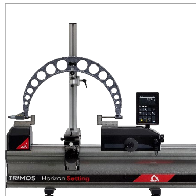
Checking of external micrometer held on a support (TA-SU-313, LABC20.1/SP02, TEL5)
