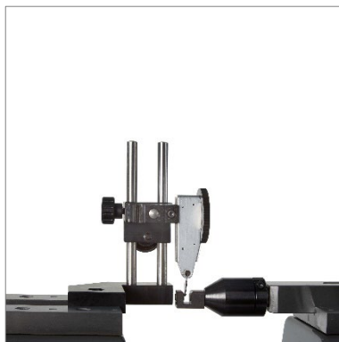
Checking of test indicators (TULM 15.1)
